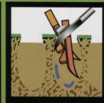
Our patented coring tine technology - combined with our planetary motion - cuts clean cores at the surface and shatters the soil below. This promotes better soil structure with less cleanup.
