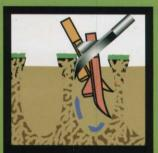
Our patented coring tine technology - combined with our planetary motion - cuts clean cores at the surface and shatters the soil below. This promotes better soil structure with less cleanup.
