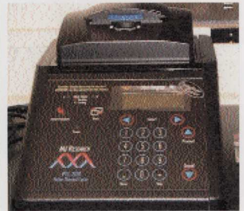
Thermal Cycler Machine
