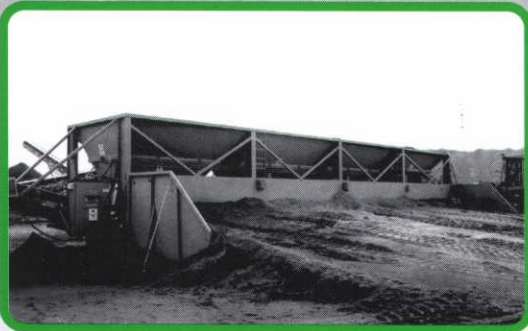
Four bin computerized blending machine with screen deck and conveyor belt.
