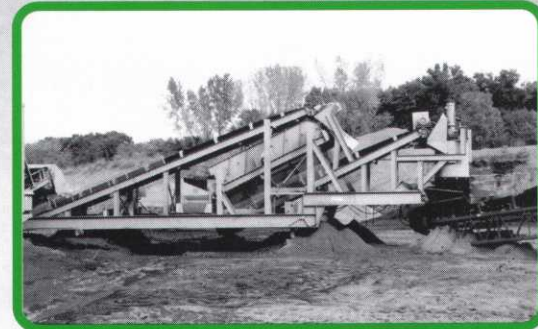
Screen deck and stacking conveyor.
