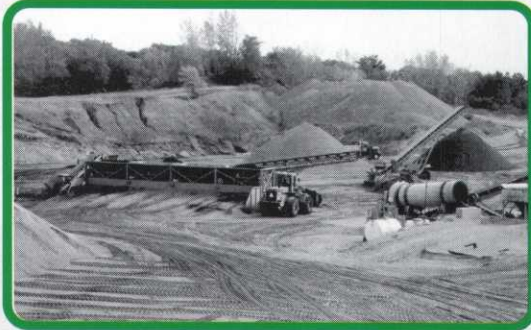
Blending yard with blender, stacking conveyor and stock piles.
