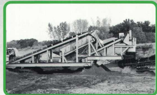
Screen deck and stacking conveyor.
