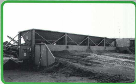
Four bin computerized blending machine with screen deck and conveyor belt.
