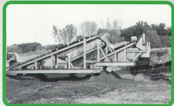
Screen deck and stacking conveyor.
