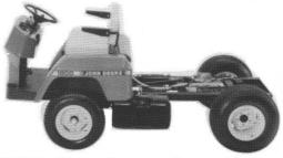
The 1800 Utility Vehicle offers tremendous work potential from one basic machine. Foot-controlled hydrostatic drive gives you an immediate advantage. Teamed with the gutsy, liquid-cooled 18-hp engine, this drive system delivers infinite speed control for precise operation. Great for jobs ranging from spraying to spreading to hauling. Other advantages include power steering, cruise control, wide stance and simple access.
