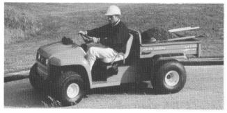
Turf Gator toughness starts with a heavy-duty, welded frame with unibody construction. Turf Gator quietness comes from an isolation-mounted engine, large volume muffler and internal sound-absorbing material — allowing you to work without disturbing play. Like a golf cart, you simply press a pedal to start and accelerate. High-flotation tires allow the Turf Gator to work hard without scuffing the turf.
