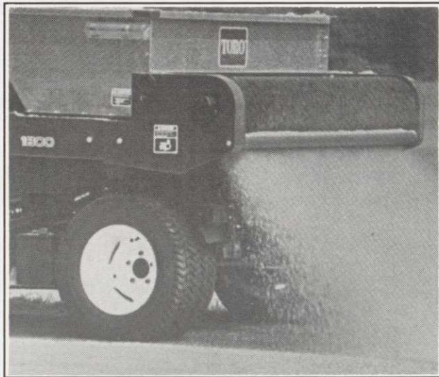
**THE TORO TOPDRESSER 1800** is a Workman™ 3000 Series attachment with PTO powered hydraulic system that greatly reduces maintenance problems, evenly distributes topdressing with a high speed brush and includes a continuous belt feed with on/off switch at the operator's position. Add the optional electric gate control and the application can be controlled from the operator's position.
