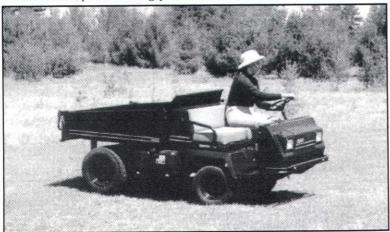
TASKFORCE XL (below) Easy operation and extended 6 1/2 ft cargo bed length. Features 2000 lb total load capacity, Kohler 18 hp OHC engine, variable speed drive, power steering, automotive-type rear disc brakes, front drum brakes.
