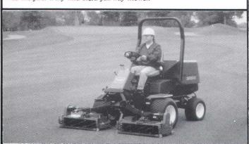
**REELMASTER® 3500-D.** (above) A versatile, hard-working triplex mower. Deisgned to mow a wide range of turf areas — hills, formal and informal turf.
