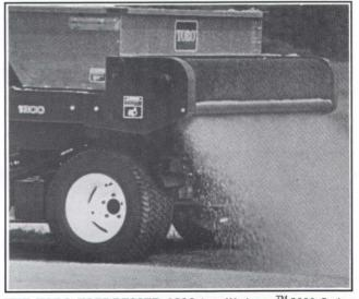
**THE TORO TOPDRESSER 1800** is a Workman<sup>™</sup> 3000 Series attachment with PTO powered hydraulic system that greatly reduces maintenance problems, evenly distributes topdressing with a high speed brush and includes a continuous belt feed with on/off switch at the operator's position. Add the optional electric gate control and the application can be controlled from the operator's position.
