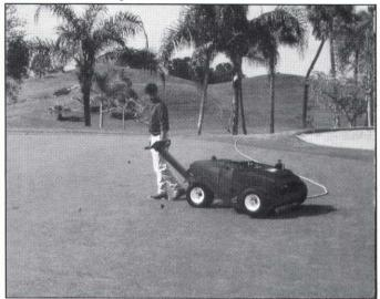
A revolutionary turf cultivation tool that deeply aerates compacted soils without causing surface disturbance using high velocity water.
