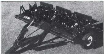
Three independent coring heads follow the ground contour both vertically and horizontally over uneven turf conditions. You get deep penetration with twelve (12) 70 lb. castings spread across a  $6\frac{1}{2}$  foot aerating swath for those large turf area jobs.
