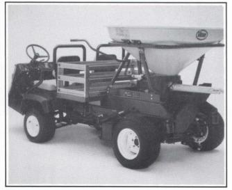
**THE WORKMAN WITH SPREADER** provides more flotation with less compaction. Toro's transaxle delivers power to the rear 23" high, 10" wide flotation tires or optional 13" wide, 24" high tires. And smooth-ribbed front tires with 70° power steering geometry practically eliminates turf scuffing or skating — even on greens, fully loaded.
