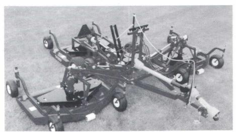
maintenance requirements are all All functions for transport and mowing positions are activated without leaving the built-in features of this mower. tractor seat.
