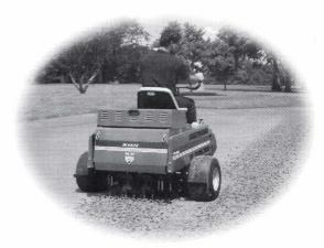
$GA^{16}$  30 —A combination of variable core spacing, speed, and precision coring. Aerate greens, tees and fairways up to a depth of 3.75 inches.
