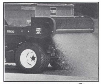
THE TORO TOPDRESSER 1800 is a Workman ™3000 Series attachment with PTO powered hydraulic system that greatly reduces maintenance problems, evenly distributes topdressing with a high speed brush and includes a continuous belt feed with on/off switch at the operator's position. Add the optional electric gate control and the application can be controlled from the operator's position.
