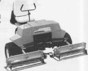
be switched from fixed to floating simply by removing a bolt. Plus, foot-operated reel lift allows the operator to keep both hands on the responsive steering yoke for fast, precise cross-cutting.
