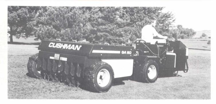
he GA 60 Aerator has proven to be more effective than any competing tractor-pulled reciprocating fairway aerator on the market. Features such as twin aerating heads, its own source of power, and floating turf guards deliver greens-caliber aeration even on undulating terrain. The heavier and beefier aerating heads provide greater strength to cover a broader range of turf conditions.
