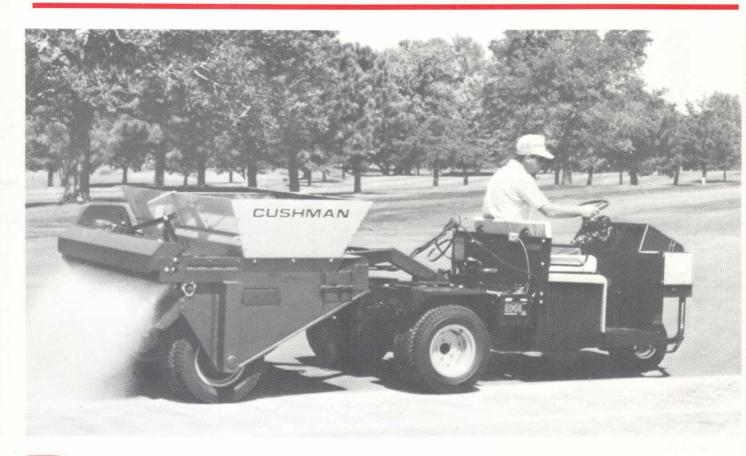
his large-capacity implement can help you save time by cutting big jobs down to size. Its 20 cubic foot hopper can hold up to 2500 pounds of material. Yet, because Cushman® never lets a detail go unattended, the weight is evenly distributed to minimize compaction. It exerts a very low 12 psi ground pressure.
