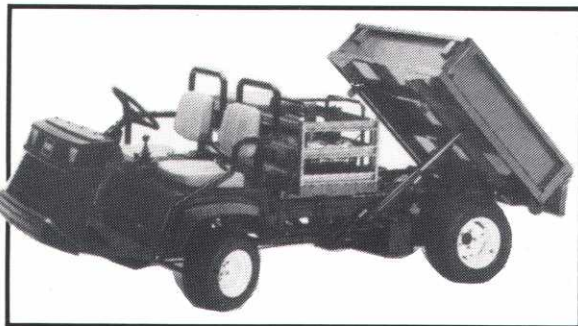
1/3 Bed with Stake Sides and 2/3 Dump Box
