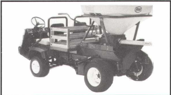
Workman with Spreader
