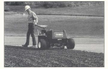
Compare that to the competition. Toro keeps you way out in front because of its increased ground speed—and wider coring width. 13,000 square feet per hour means you'll do the job almost twice as fast as you're doing it today.
