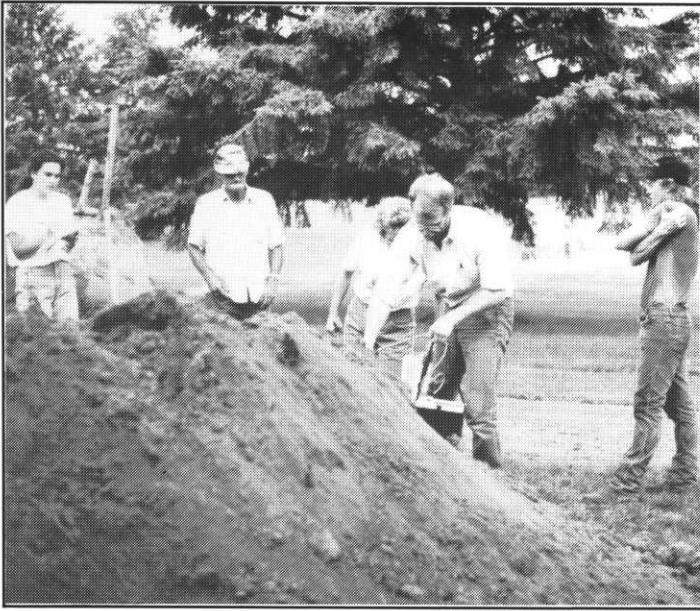
Peter Sandberg of Twin City Testing uses a photoionization detector in the stockpile of contaminated soil.
