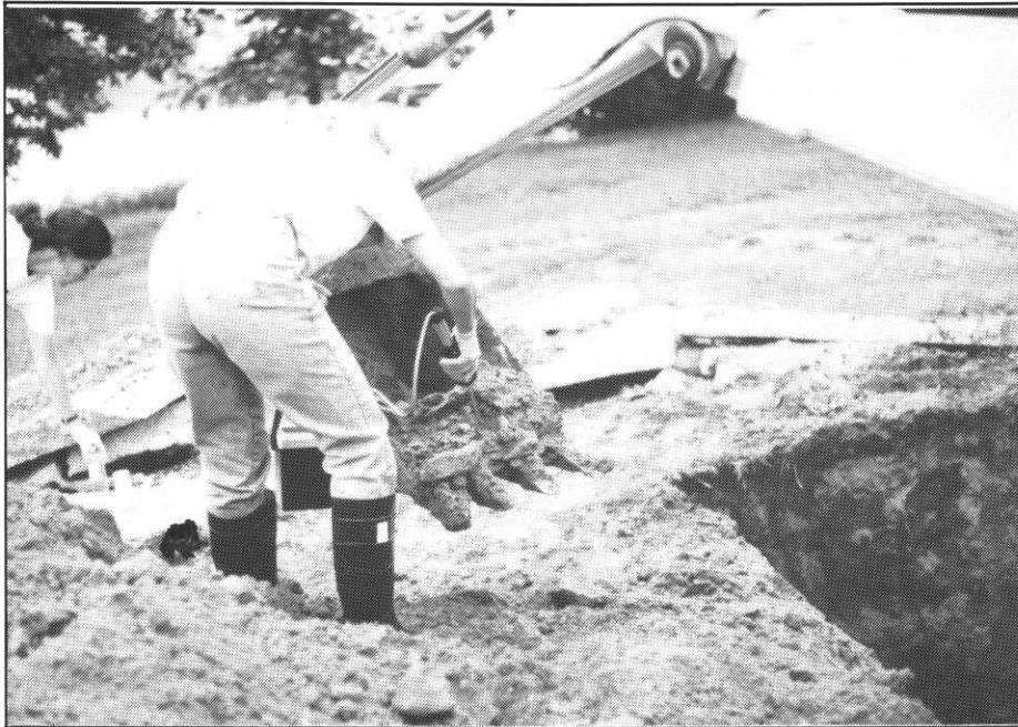
Technician checks for contamination on the final scoop from 12 feet below ground level.
