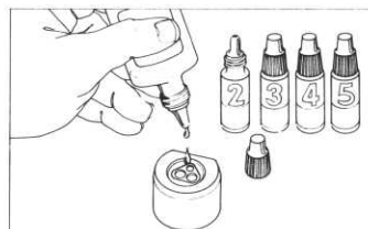
Remove a disease detector from its pouch. Squeeze drops of test solutions onto the detector in sequence.
