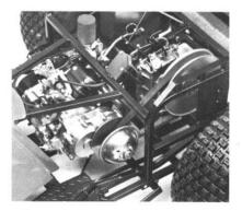
The 1200 Bunker and Field Rake features a Kawasaki 10 hp, 4 cycle, air cooled, overhead valve engine with full pressure lubrication and a standard oil filter.
