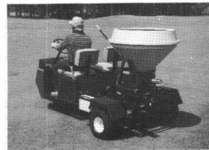
GXT-1500 with seeder spreader.
