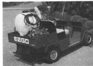
XT-500 with bed mounted sprayer.
