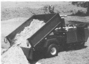
GXT-1500 with hydraulic dump.
