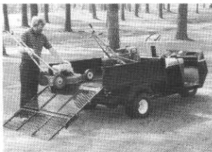
GXT-1500 with loading ramp.
