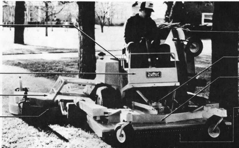
Twin lever steering and dual hydrostatic drive make the Range Wing highly maneuverable.
