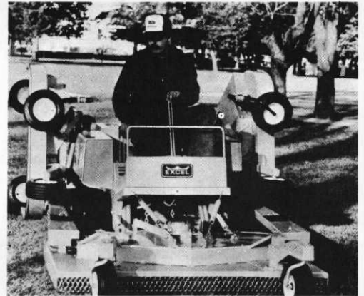
Twin lever steering and dual hydrostatic drive make the Range Wing highly maneuverable.
