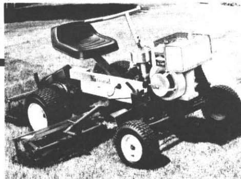
MODEL 68: Standard B&S, 1/C, heavy duty engine. Three powered reels provide 68" cut.
