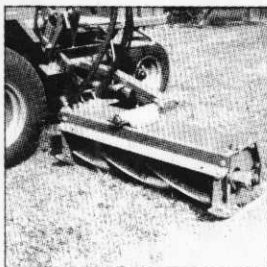
6 or 8 knife fixed or floating cutting units for any and all mowing conditions.
