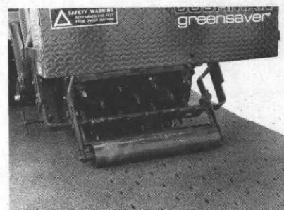
The Greensaver delivers a precise 3¼" x 4" pattern of aeration.
