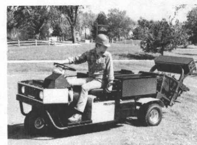
With the optional live hydraulics system, you can raise or lower the Greensaver as you work.
