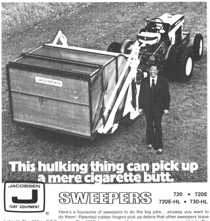
behind! The 720 is P.T.O. driven. The 720E has its own 12 h.p. engine and a universal hitch. The 720E-HL has engine plus hydraulic lift dumping. The 730-HL is a P.T.O. sweeper that dumps hydraulically. Whichever you choose for your turf, you have a sweeper that sweeps wet or dry for positive removal of grass clippings, leaves, branches, cans, rocks, and other debris. The "Clean-Sweep" program is underway with a Jacobsen Sweeper in your fleet!
