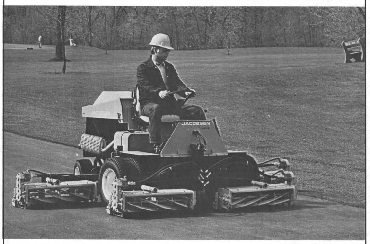
HERE IS JACOBSEN'S NEW HF-5...A COMPACT HYDRAULIC MOWING TRACTOR THAT'S THE FIRST MACHINE IN ITS CLASS WITH DIESEL POWER.
