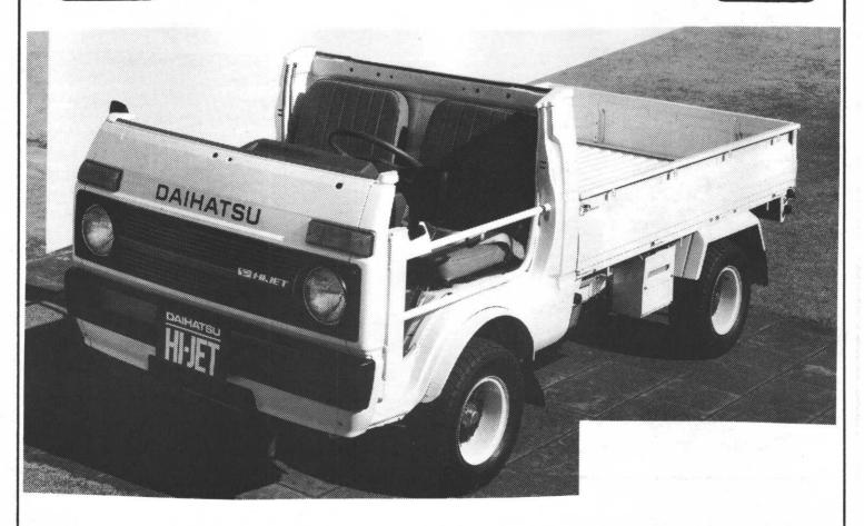
ENGINE WATER-COOLED, 2 CYLINDER, 4 CYCLE
