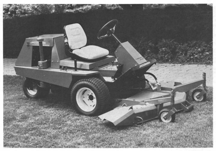
THIS NEW JACOBSEN MID-SIZED, OUT-FRONT RIDING ROTARY MOWER FEATURES HYDRAULICALLY DRIVEN CUTTER BLADES DIESEL POWER AND THE ABILITY TO HANDLE A VARIETY OF IMPLEMENTS THAT EXTEND ITS UTILITY THROUGH ALL SEASONS. THE TURFCAT II DW 220 IS CAPABLE OF MOWING UP TO 24 ACRES OF TURF IN AN AVERAGE WORKING DAY WITH ITS 72-in. SIDE-DISCHARGE DECK. IT IS ALSO AVAILABLE WITH 60-in. REAR- OR SIDE-DISCHARGE DECKS, OR A 60-in. FLAIL MOWER AND SNOWTHROWER, PLOW AND ROTARY BROOM ATTACHMENTS.
