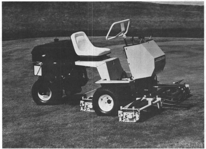
AN ALL-HYDRAULIC MACHINE, THE NEW JACOBSEN TRIM KING CUTS A 70" SWATH AND HAS A FRONT MOWER OVERHANG OF 10" NEGOTIATING SAND TRAP EDGES, CURBS AND SIMILAR MANEUVERS. POWERED BY A 16 HP AIR-COOLED ENGINE, THE MACHINES HYDRAULICS PROVIDE VARIABLE TRACTION SPEED AND DUAL ROTATION, AS WELL AS POWER FOR RAISING AND LOWERING UNITS. POLYETHYLENE CATCHERS AVAILABLE.
