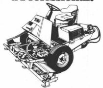
The Toro\* Turf Pro 84 is an all hydraulic triplex that gives you the right clip for the right height of cut and type of grass. All three reels and wheels are hydraulically powered, reducing maintenance time and cost. Reels have independent suspension, providing a better quality of cut. With movement of a single pin, cutting height adjusts from %" to 2½." Front rollers, grass catchers and delive series are optional.
