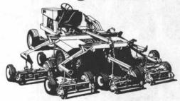
The Toro' Parkmaster mows swaths from 30 inches to 18½ feet wide —up to 80 acres a day. With a 7 or 9 unit hydraulically-controlled frame, it has a compact pattern of gangs for easy mowing, easy transporting. The Parkmaster is the mowing tractor built to take Spartan' gangs. Comes with
