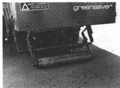
The Greensaver delivers a precise 3½" x 4" pattern of aeration.
