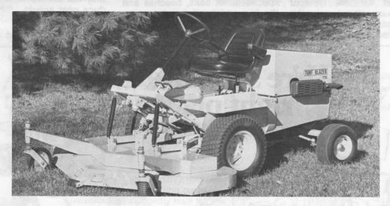
The Turf Blazer 727 with its 27 H.P. Yanmar liquid cooled <u>Diesel</u> engine and 72" cutting head combines diesel lugging power, durability and fuel efficiency with the trimming capabilities of an out front offset deck.
