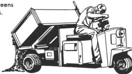
DUMPING/HAULING 1000 lb. payloads. Manual and hydraulic dumping.
