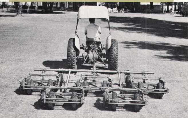
Roseman Rubber-tire mowers improve fairways. Rear drive design eliminates bobbing for smooth, uniformly cut, perfect playing surfaces.
