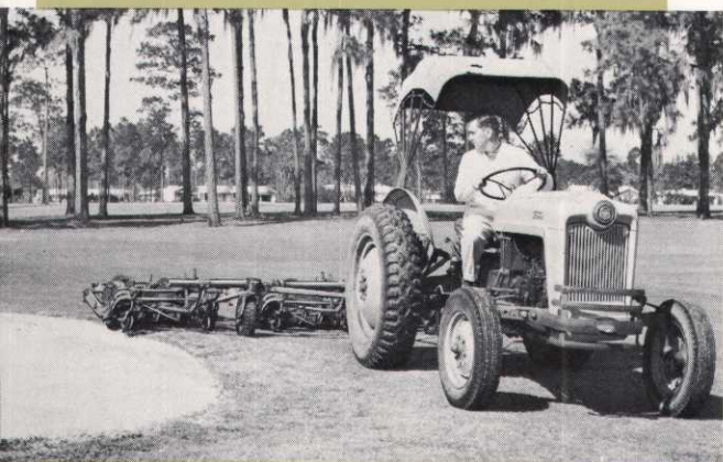
Only ROSEMAN mowers can overhang traps and shrubbery beds without drop off. Exclusive rear drive design supports reel over edge. No unsightly fringe remains for costly hand trimming. Appearances improved at no extra cost.
