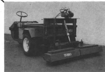
WORKMASTER WITH SPIKER HYDRAULIC DOWN PRESSURE
