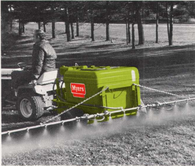
Optional TLT Trailer with Terra Tires converts Myers skid cart sprayers to trail behind riding lawn tractors or turf carts. TLT trailer complete with hitch, foot standard and 4 ply 18 x 9.00 x 8 Terra Tires.
