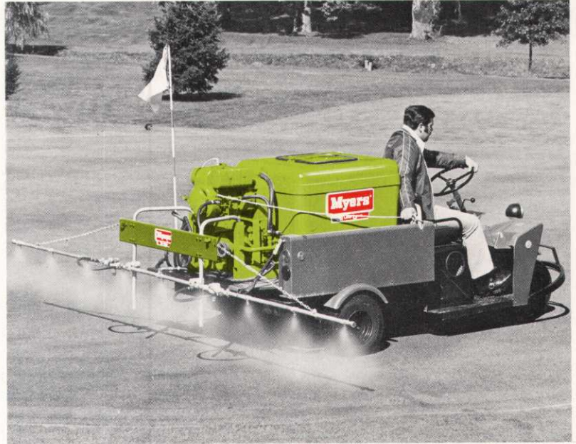
Custom designed sprayers with choice of 40 GPM – 30 PSI or 10 GPM – 300 PSI performance range. Optional anchor kits to fit Toro Workmaster, Otis Westcoaster, E-Z-Go Maintenance Machine and other utility carts. Lightweight, easy to install and remove. Optional gun for spraying trees and shrubs.
