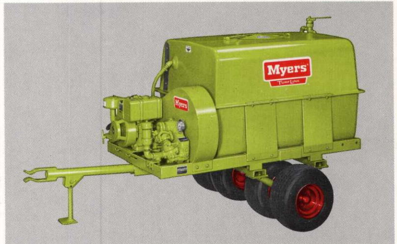
The VTL10 series sprayers are available for fairway and general turf maintenance in trailer or skid models and feature 200 gallon fiberglass tanks. Pump has 10 GPM – 500 PSI performance range. Powered by 7 HP single cylinder, 4 cycle air cooled engine or PTO drive. Unit pictured shows optional dual wide track running gear with Terra Tires (regularly furnished with wheels for 15" tires).
