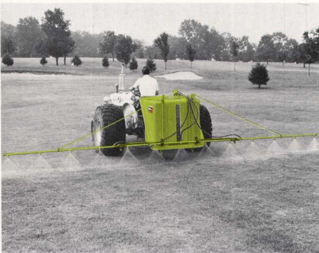
TL12TMG tractor mounted sprayer with economical PTO drive. Basic sprayer has 100 gallon fiberglass tank, 12 GPM – 500 PSI performance range. Optional 21' galvanized boom has 13 Teejet nozzles spaced 20" apart. 6 GPM – 300 PSI model also available.
