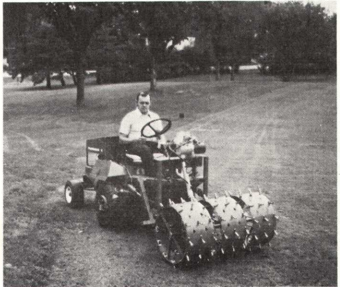
GLENN RASMUSSEN, GENERAL MANAGER AND VICE-PRESIDENT OF TURF PRODUCTS DIVISION OF MINN. TORO, OPERATING A DEDO AERIFIER MOUNTED ON A 72" TORO GROUNDS MASTER POWER UNIT.
