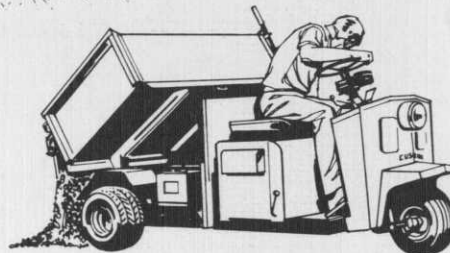
DUMPING/HAULING 1000 lb. payloads. Manual and hydraulic dumping.
