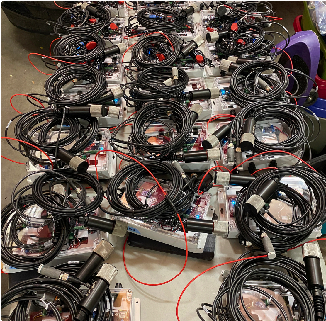
Figure 2: The GEMS sensing group at the University of Minnesota designed environmental nodes that are collecting millions of data points all winter long on golf greens in the United States, Canada, and Europe. Photo credit: Andrew Hollman.
