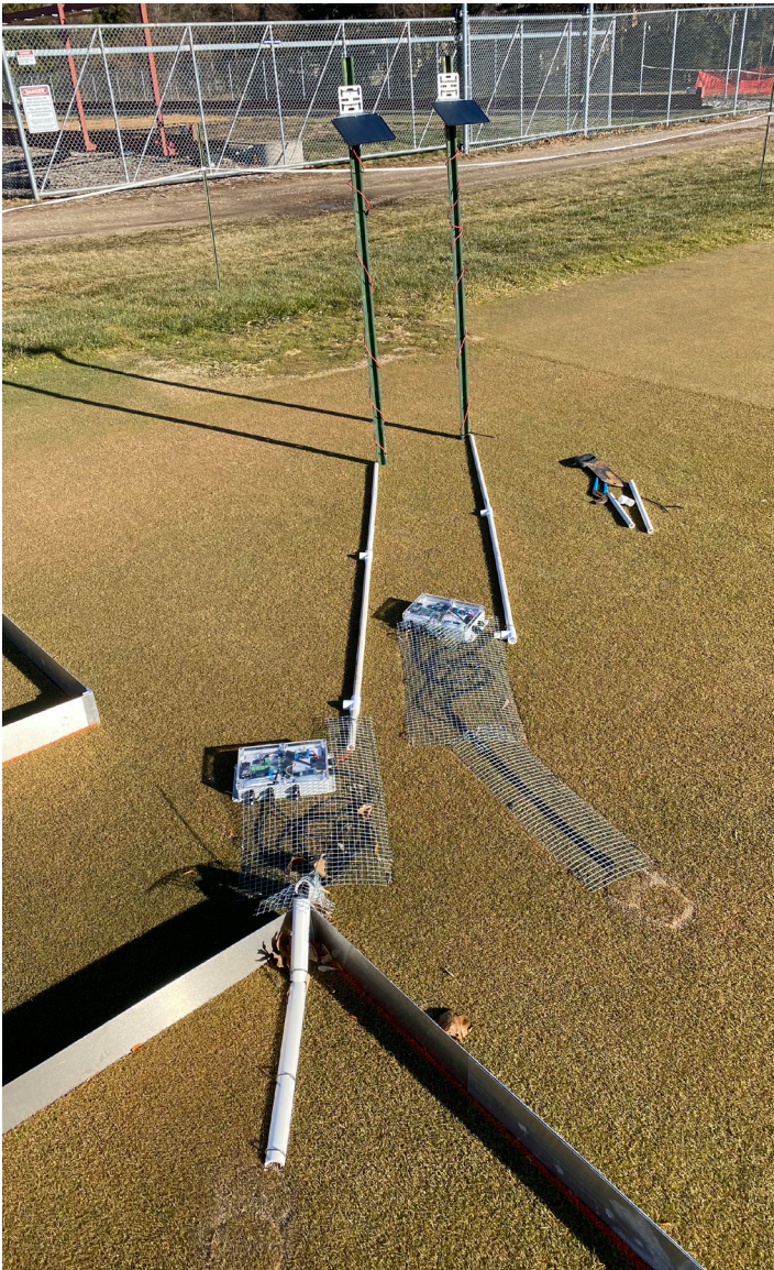
Figure 1. Sensor nodes installed on the trial with coverings to protect from coyote damage
