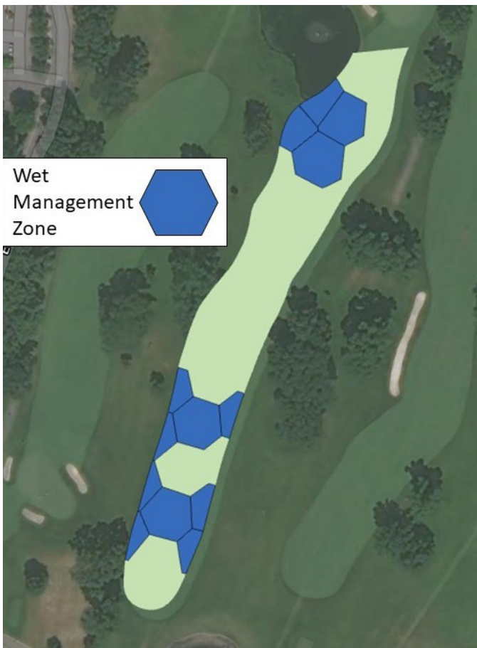
Figure 1. Locations of a “wet” irrigation management zone based on soil moisture mapping of a fairway.
