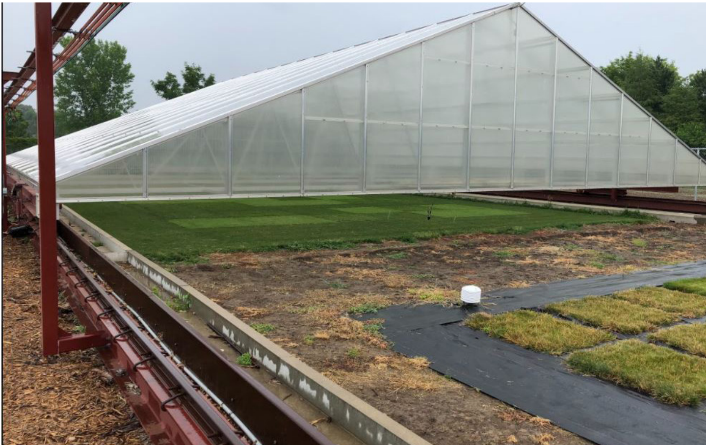
Figure 2. The rainout shelter hovered over the plots during rain events while dry downs were occurring. Photo credit: Josh Friell
