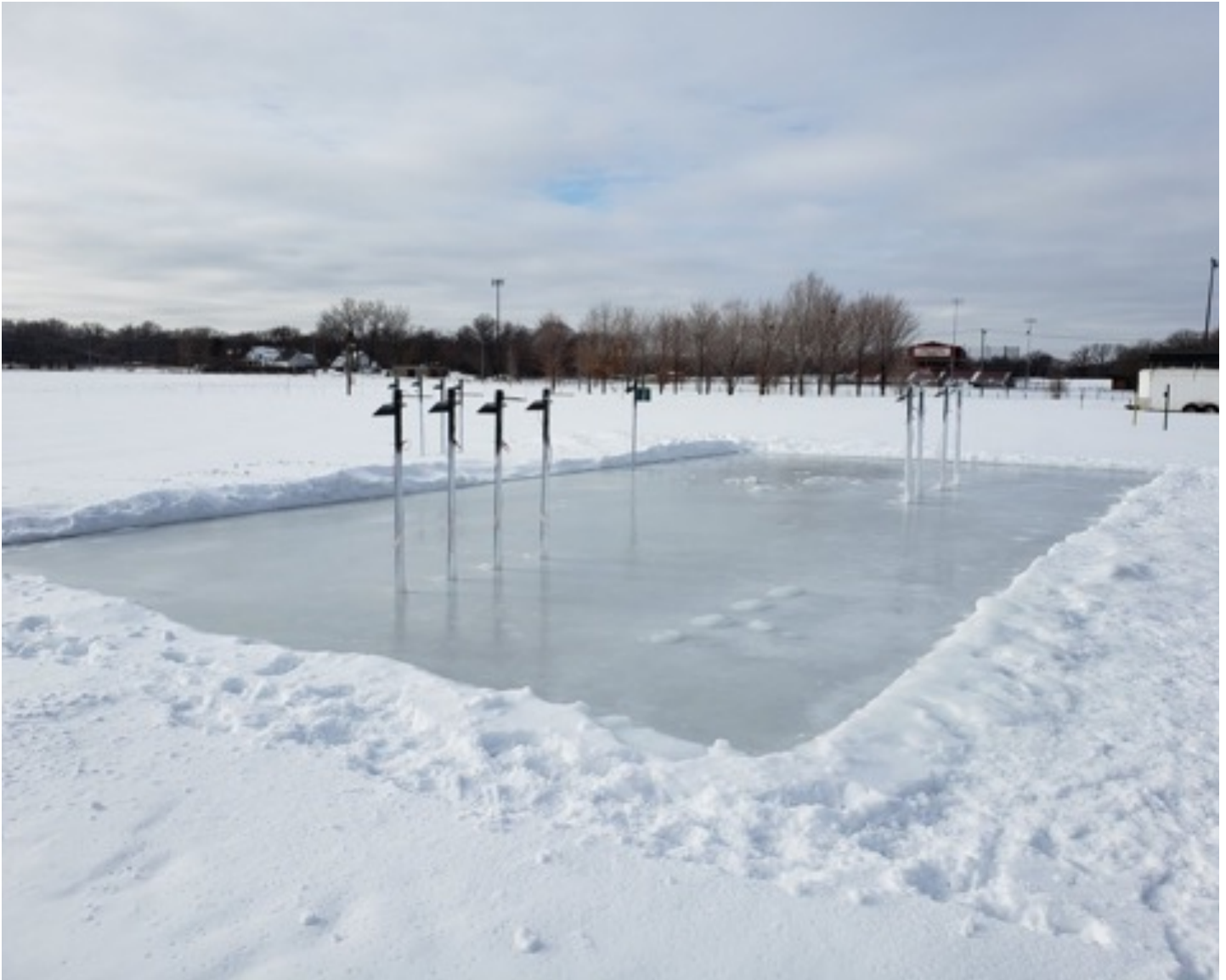
Figure 2. Sensors set up in St. Paul where they were deliberately encased in ice.
