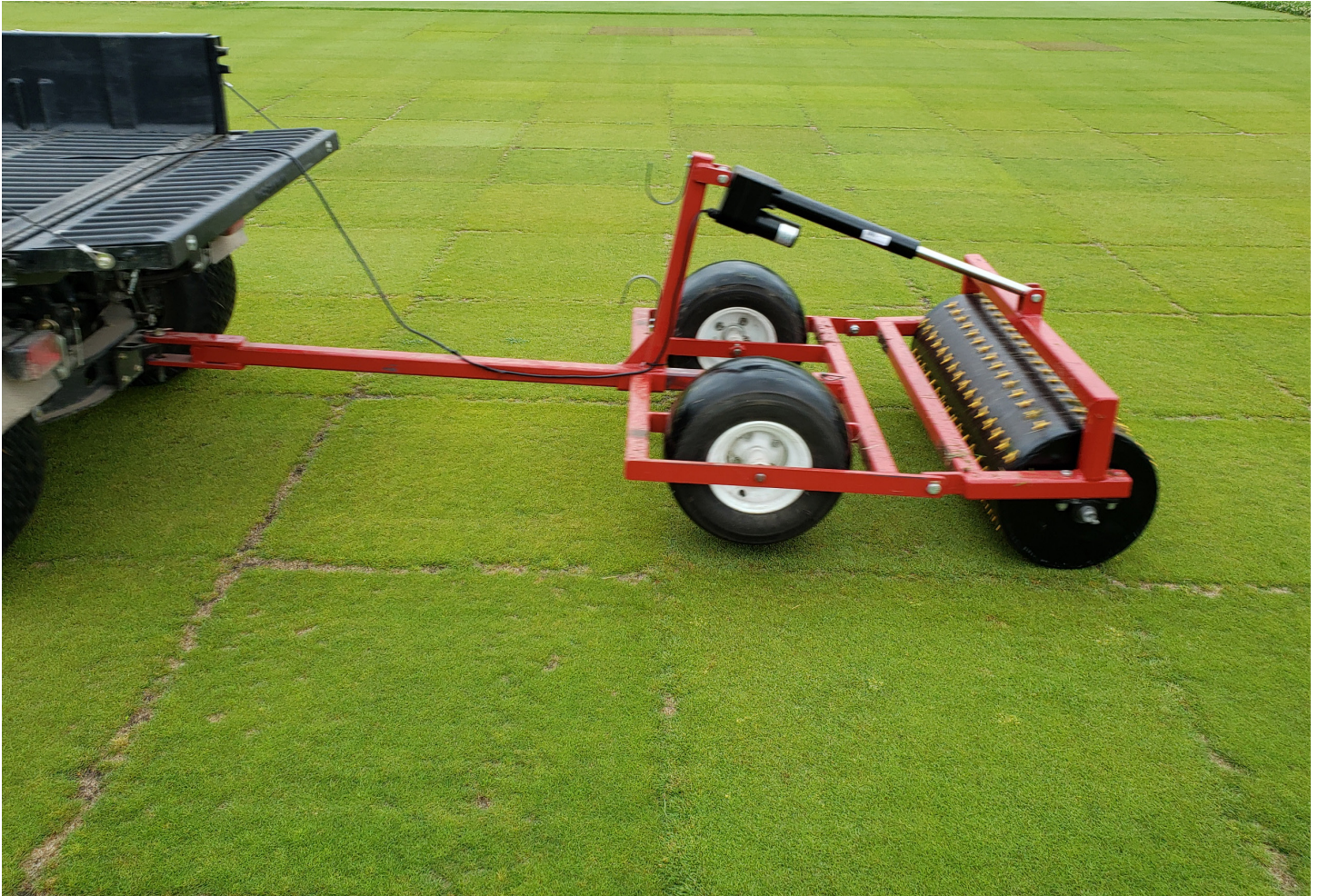
Figure 3: Beginning in mid to late June, the entire SCANGREEN plot area receives traffic application using this device each Tuesday and Thursday, with the device making three passes over the plots each day.
