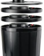
Over time, the application of topdressing and settling can result in the sprinkler being in a depression below grade level. This can interfere in the natural roll of the ball, create trip hazards and take away from the natural beauty of the course. The Razor kits are designed to raise the top of the sprinkler in ½" increments up to 1½" (3 stages) without digging!
