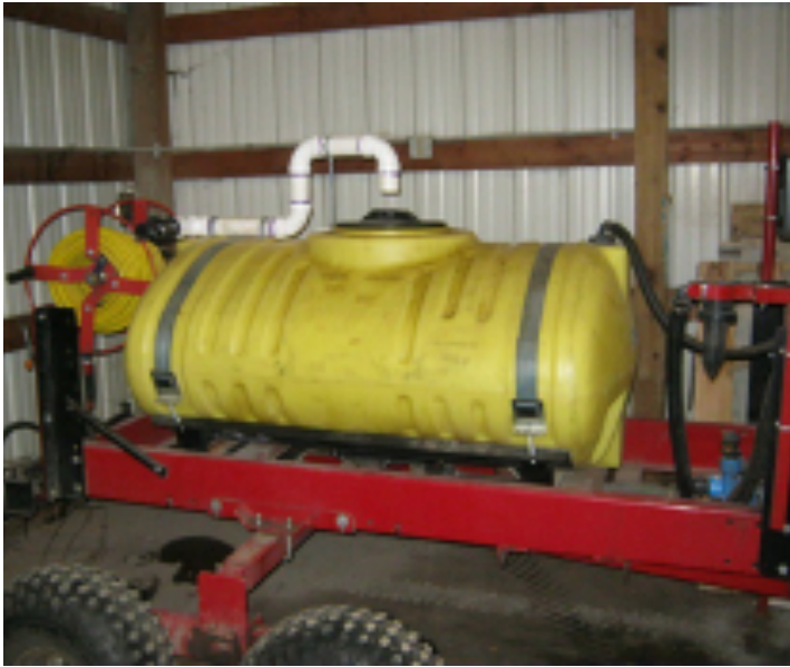
Above and on the left, a fixed and ridged air gap. On right, a removable fixed air gap device.
